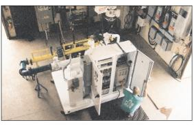
Each pumping system is dynamically flow tested in our factory prior to shipment. Mechanical, electrical and control systems are put through their paces and a full report is logged into the station records.
